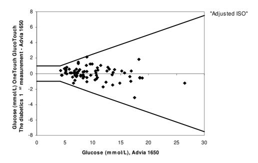
Figure 3. Accuracy. The diabetic patients' self-measurements at the final consultation. Three lots of test strips. The x-axis represents the mean value of the duplicate results at the comparison method. The y-axis shows the difference between the first measurement at OneTouch GlucoTouch and the mean value of the duplicate results at the comparison method. N = 76.
