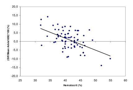
Figure 5. The effect of hematocrit at glucose measurements on OneTouch GlucoTouch under standardised and optimal conditions. The x-axis shows the hematocrit value in %. The y-axis shows the difference in glucose concentration between OneTouch GlucoTouch and the comparison method (OneTouch GlucoTouch – the comparison method) in percent. n=77
