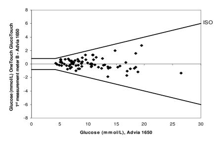
Figure 2. Accuracy. One Touch Gluco Touch meter B (three lots of test strips) under standardised and optimal measuring conditions at the final consultation. The x-axis represents the mean value of the duplicate results at the comparison method. The y-axis shows the difference between the first measurement at One Touch Gluco Touch and the mean value of the duplicate results at the comparison method. N = 78.
