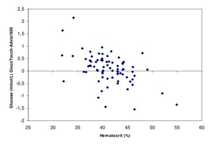
Figure 4. The effect of hematocrit at glucose measurements (in mmol/L) at OneTouch GlucoTouch under standardised and optimal conditions. The x-axis shows the hematocrit value in %. The y-axis shows the difference in glucose concentration between OneTouch GlucoTouch and the comparison method in mmol/L. n= 77
